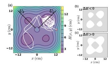
FIG. 2. (a) A typical experimental trajectory, shown in white, on the potential energy surface where the contours denote isoheights of the surface. This instance of the trajectory was traced by the ball released from rest, marked by a red cross. Parts (b) and (c) show the energetically accessible region projected on the configuration space in white for  $\Delta E < 0$ :  $\Delta E = -100 \text{ (cm/s)}^2$  and  $\Delta E > 0$ :  $\Delta E = 100 \text{ (cm/s)}^2$ , respectively.
