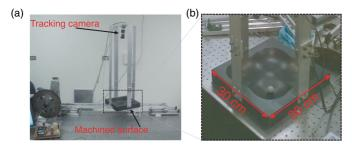
FIG. 5. (a), (b) Experimental apparatus showing the machined surface, tracking camera, and the rubber coated steel ball.
