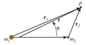
Fig. 2.1. The relationship between distances in the restricted three-body problem.
