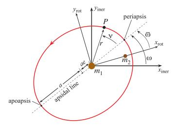
FIG. 2.2. The osculating or instantaneous orbital elements for a particle P in a near-Keplerian orbit about a massive central body  $m_1$ . The perturbing body,  $m_2$ , is in a circular orbit about  $m_1$  of unit frequency and the x axis of the rotating frame is defined as the line from  $m_1$  to  $m_2$ , where the y axis of the rotating frame completes a right-handed coordinate system.
