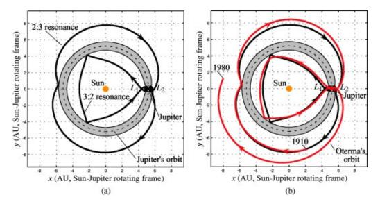
FIG. 32. (Color online) (a) The homoclinic-heteroclinic chain corresponding to the Jupiter comet Oterma. (b) The actual orbit of Oterma (AD 1910–1980) overlaying the chain.
