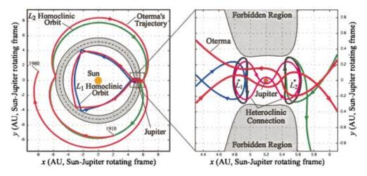
FIG. 2. (Color) A dynamical channel (homoclinic–heteroclinic chain) corresponding to the Jupiter comet *Oterma*. The periodic orbits about  $L_1$  and  $L_2$  are black. Their homoclinic orbits are blue and green. The heteroclinic connection between them is magenta. The actual orbit of *Oterma* (AD 1910–1980) is shown in red overlaying the chain. Distances are in Astronomical Units (AU).
