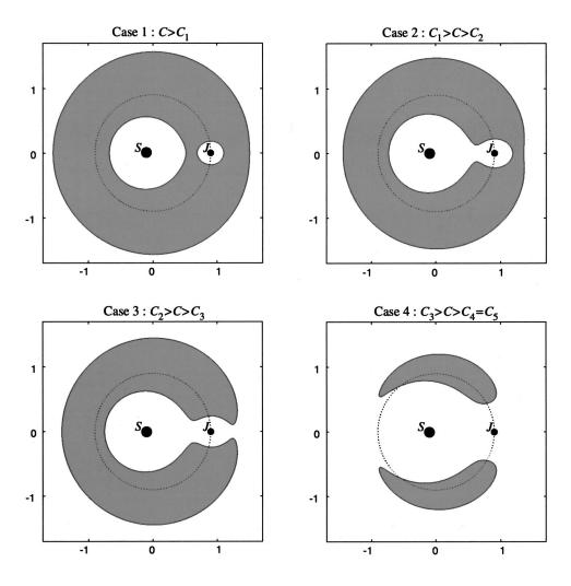
FIG. 10. Four basic configurations of the Hill's region.
