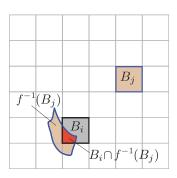
FIG. 5. Computation of the transition matrix  $P_{t,\tau_j}$  by a set-oriented method. The phase space is divided into boxes,  $\{B_1, B_2, ..., B_n\}$ . Box  $B_j$  at the final time  $t + \tau_f$  is mapped (backwards) to  $f^{-1}(B_j)$  at the initial time t, where  $f = \phi_t^{t+\tau_j}$ . The value of the entry  $p_{ij}$  is the fraction of box  $B_i$  that is mapped into box  $B_i$  by f.
