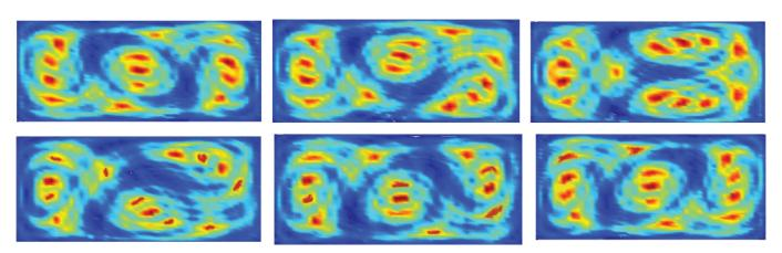
FIG. 12. AIS identified by second eigenvectors of time-shifted  $R_{t_i,\tau_f}$  for the first half of the flow period  $\tau_f$ , where  $\tau_f \approx 0.93$ . Left to right: Top-row:  $t_i/\tau_f = 0$ , 0.1, 0.2. Bottom row:  $t_i/\tau_f = 0.3$ , 0.4, 0.5. The braiding motion of the 13 ACS is evident, and is illustrated in Fig. 13 (enhanced online) [URL: http://dx.doi.org/10.1063/1.4768666.3].
