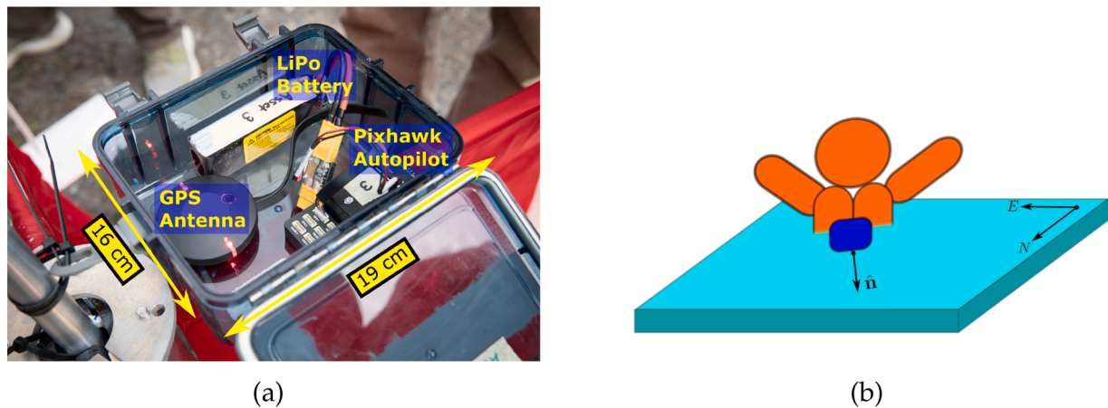
Fig. 6. a) An image of the Pixhawk-GPS module used to track search-and-rescue manikins and accompanying surface drifters. b) A schematic drawing showing the front of search-and-rescue manikins and Pixhawk-GPS modules aligned such that the orientation of each manikin be measured as the angle between the unit vector \hat{n} and North.
